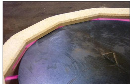
Intentional element contact with the shelf was designed to test the potential for damage from kiln element and controller electrical feedback.
