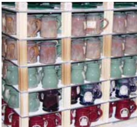
The kiln at Deneen Pottery. The company can load 100 additional pieces per firing using the 5/16-in. Advancer shelves.
