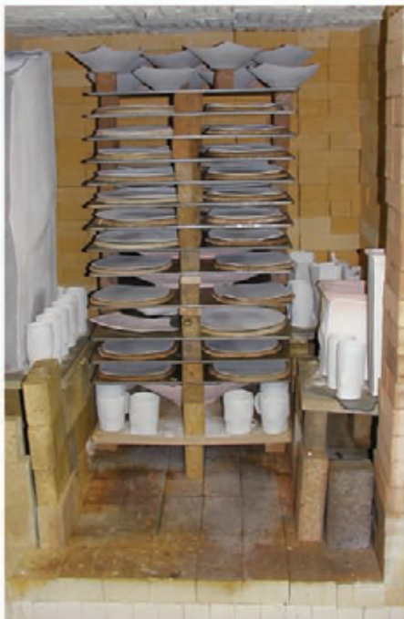
Eric's kiln loaded with ware and Advancer shelves.
