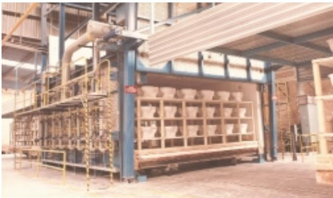
A typical traditional kiln furniture arrangement for a sanitaryware shuttle kiln.
