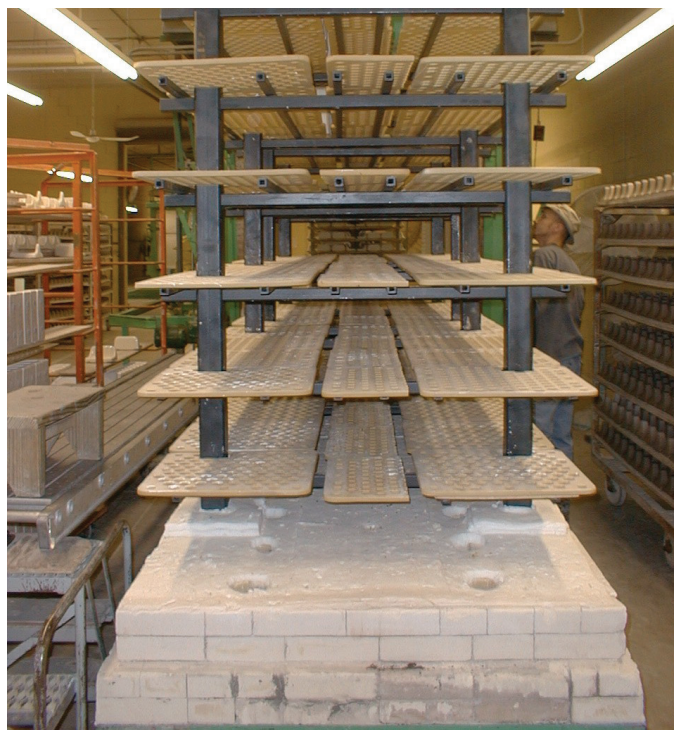
An advanced SiC kiln car using reaction-sintered, silicon-infiltrated SiC beams and posts to support perforated cordierite kiln shelves. Photo courtesy of AC products in Apple Creek, Ohio.
