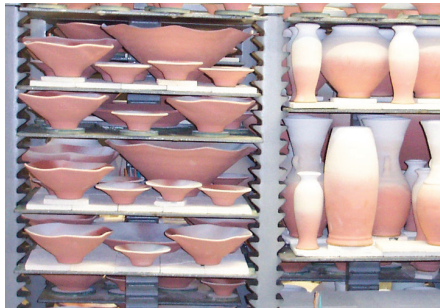
Glazed work being loaded for firing on an advanced NSiC shelf and lug post system. The ceramic barrier plates under the pots are used to contain the crystalline glaze run offs—no barrier is needed in a normal firing. Photo courtesy of Campbell Studios, Inc., Cambridge Springs, Pa.
