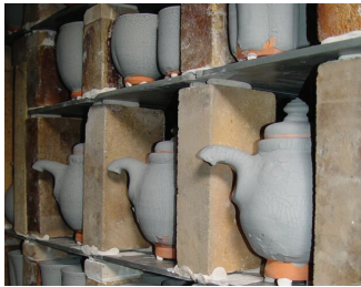
Glazed pots on advanced NSiC kiln shelves ready to be fired in a multi-chambered, wood-fired kiln. Clay wadding is used with the dense brick supports. Photo courtesy of Richard Bresnahan at Saint John's University in Minnesota.
