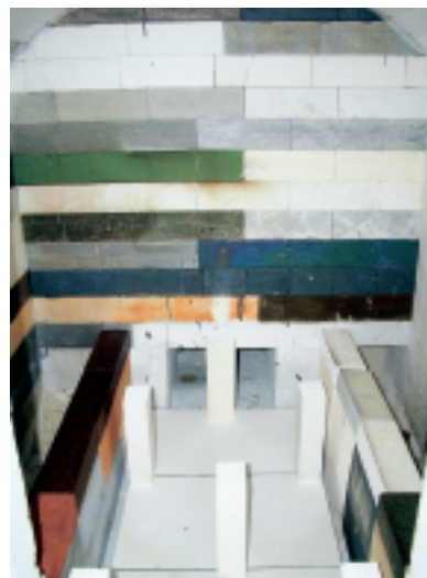
Kiln #1. Showing the exterior and interior with various bricks and refractory coatings in place.
