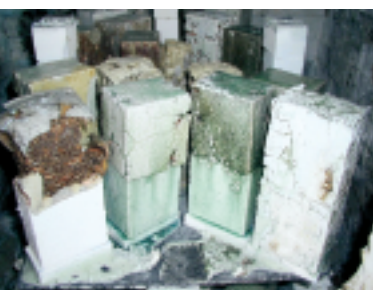
Top: and centre: Kiln #1 after salt firing 63 before dismantling. Above: Some of the new tests fired at the top level in the kiln.
