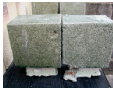
Results of tests using From the top: HD 25 brick and Furnacecoat. Calor brick and ITC, 43 firings. HD25 brick with NTE coating. Calor 26 brick and NT7 coating, 43 firings.
