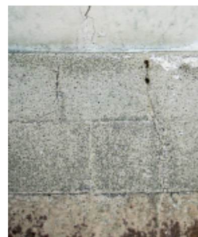
Top: Salt firing #50. Bricks HD 25 coated with NT8. Above: Salt firing #50. Caldor 26 brick, NT8 coating.
