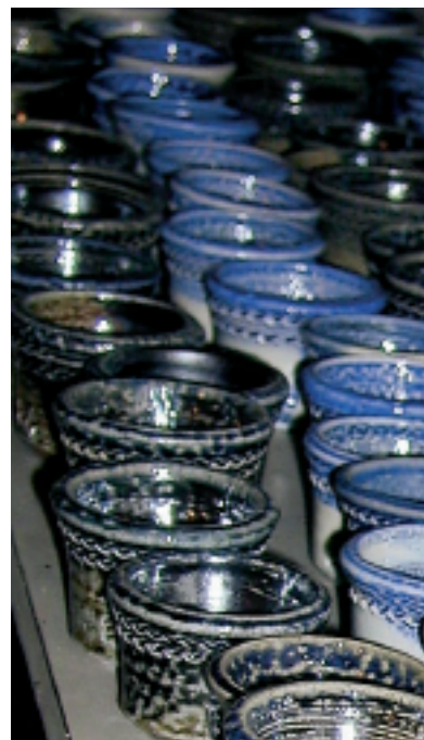
Fired body tests demonstrating effective salt-glaze throughout the kiln.
