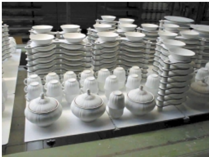
Figure 1. Fast firing tunnel kiln with SiC plate setters and batts. Photo courtesy of Saint-Gobain Ceramics and Plastics.
