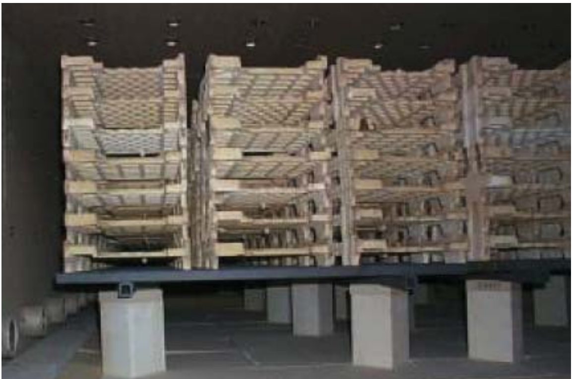
Beams made with the new N-SiC material support a car structure in a roof tile tunnel kiln.
